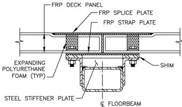
Figure 14: Deck support detail
