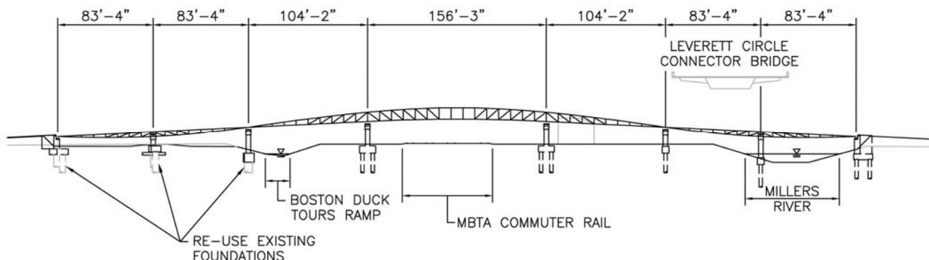
Figure 3: Elevation
