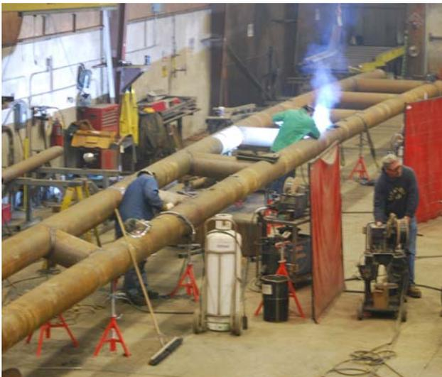
Figure 9: Truss fabrication
