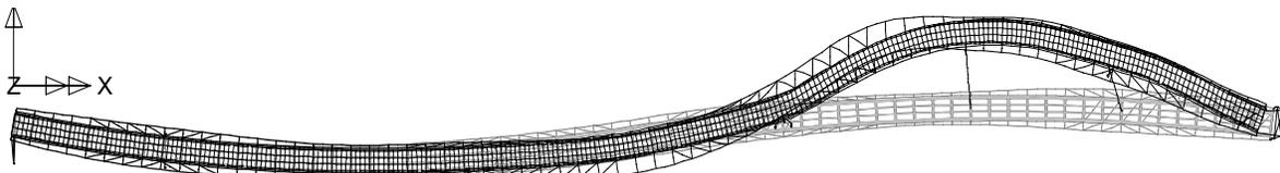
Figure 7 Plan showing first lateral mode of vibration,  $f = 1.6$  Hz
