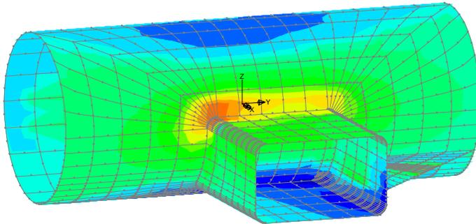
Figure 9 Shell element model of floorbeam to chord joint
