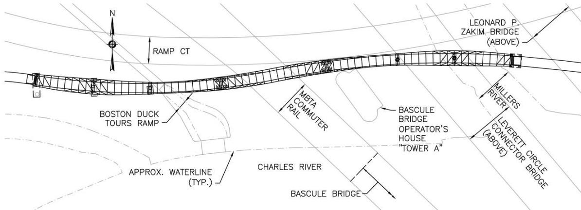
Figure 3 Plan of bridge and site
