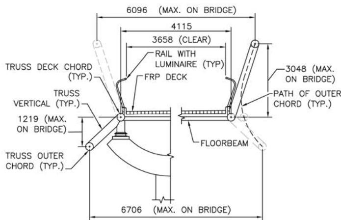
Figure 5 Typical section of bridge
