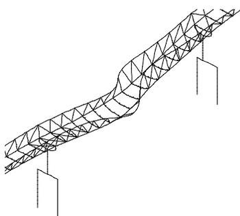
Figure 8 Detail of buckled outer chords at main span
